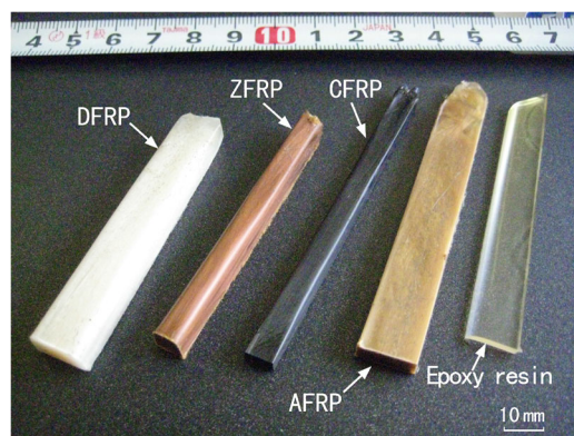
Figure 4. Specimens (from left to right) of DFRP, ZFRP, CFRP, AFRP and the neat epoxy resin. This figure is published in color in the online version.
